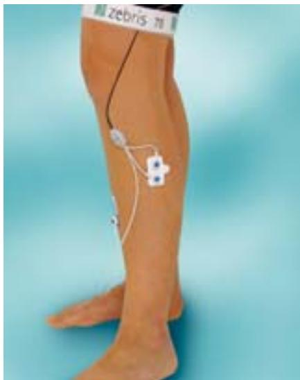
Through use of the optional bluetooth telemetry EMG, muscle function can be analyzed parallel to the floor reaction forces. By connecting goniometers it is also possible to record the angles of the joints. Up to eight analog signals can be synchronized to the force values and displayed in the evaluation software.
