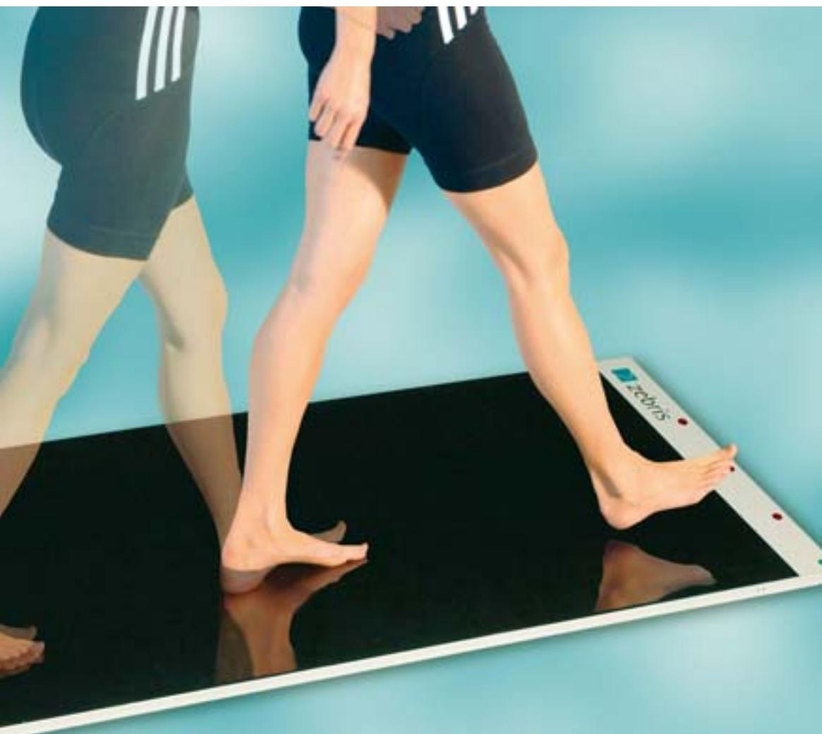
The measuring plate is integrated in a level walking area and can also be used with walking aids. The measuring cycle can be repeated up to four times. The measuring parameters are automatically calculated in the software program.
