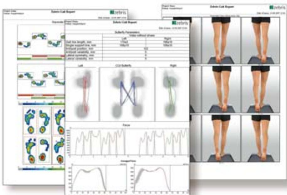
In other analyses, gait symmetry is assessed in addition to gait lines, standardized and averaged force variation curves. Besides of maximum pressure plots complete videosequences can be displayed.
