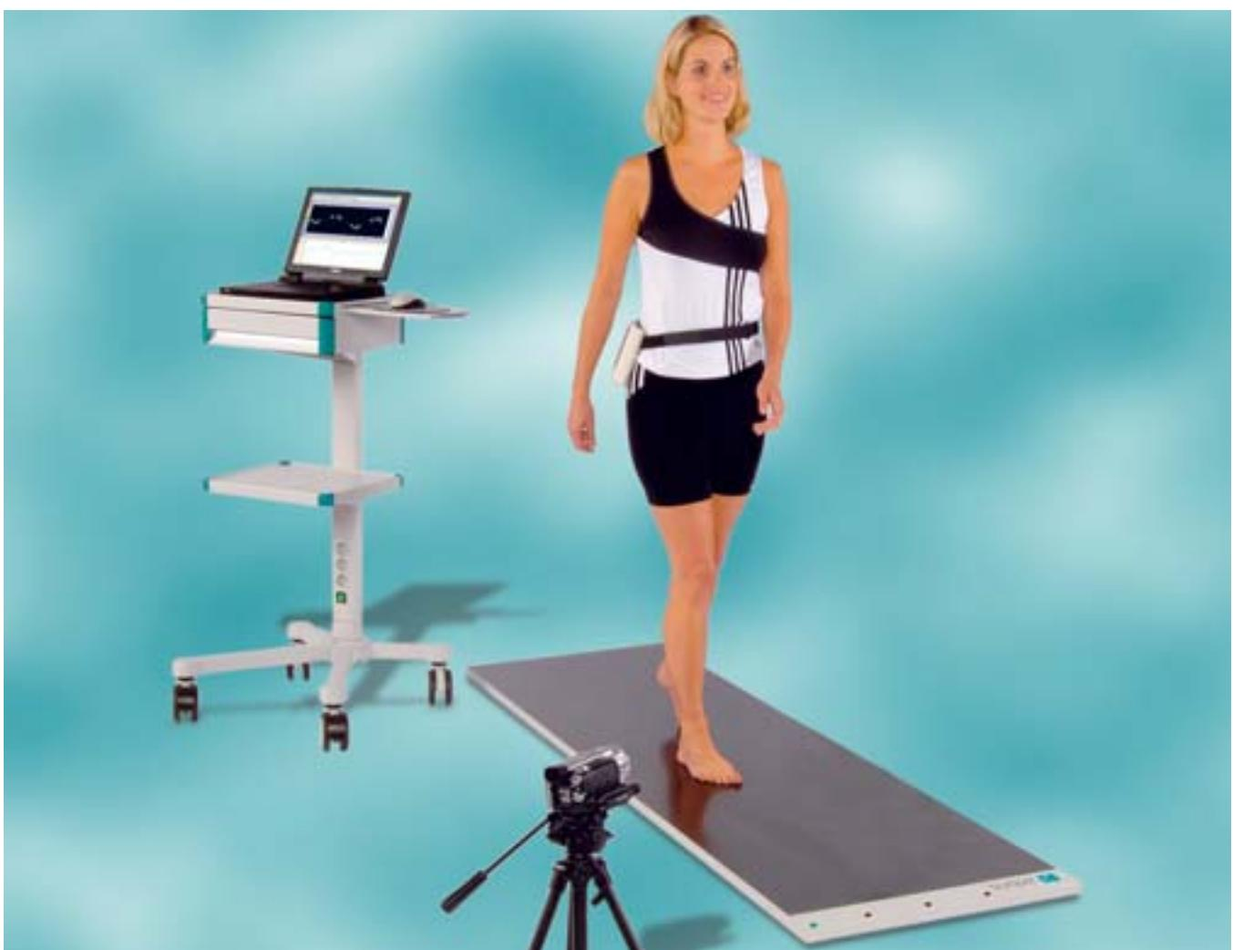
The basic measuring system comprises a measuring plate FDM 1.5, FDM 2 or FDM 3, an external power pack and the WinFDM software package. The system operates using a PC with USB interface and the Windows XP / Vista operating system.
