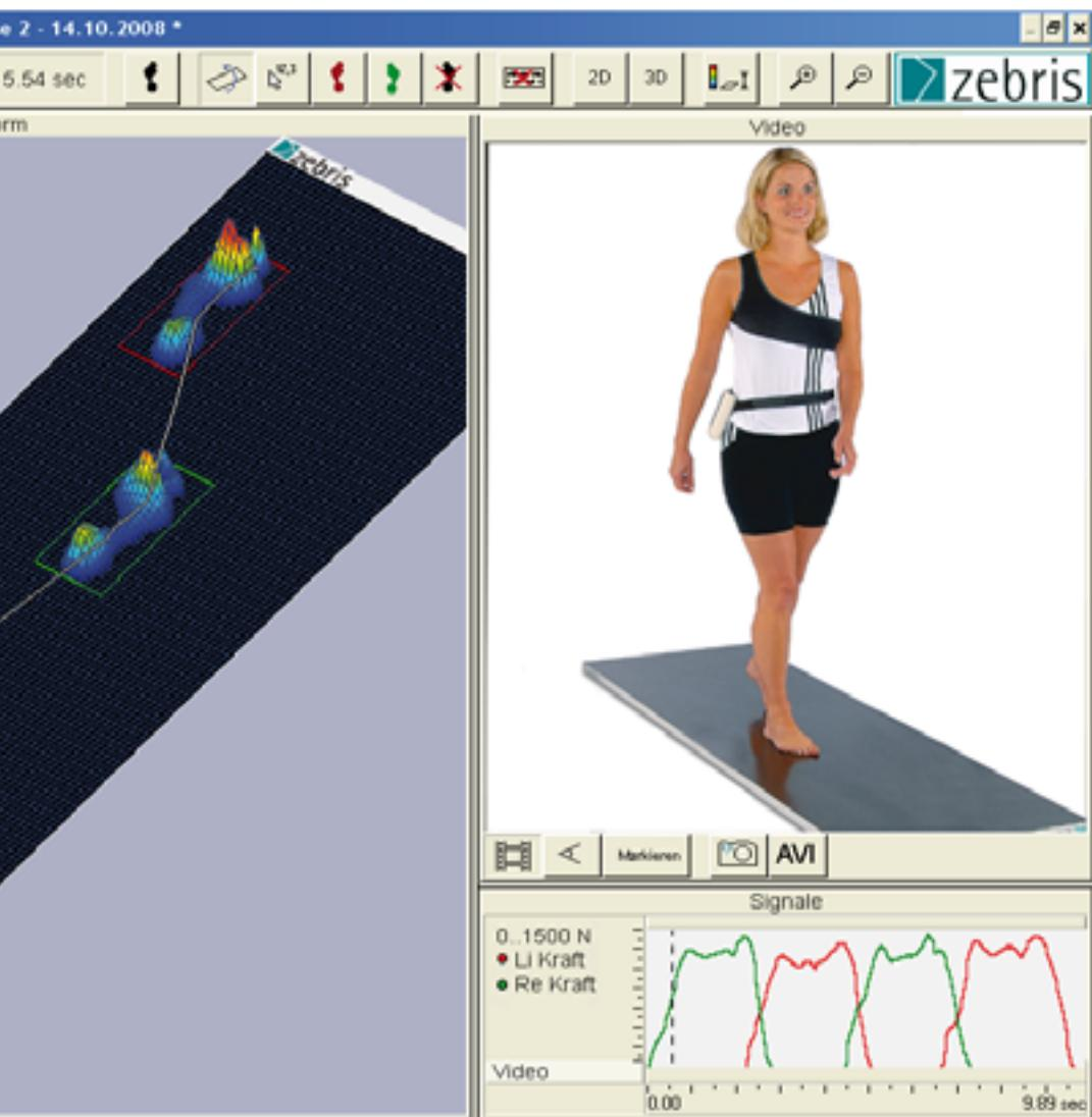
On the measuring screen and viewer the image of the measuring plate can be altered three dimensionally. Also the image size can be reduced or enlarged as required. Force variations, video images, EMG and angle data may also be displayed simultaneously.
