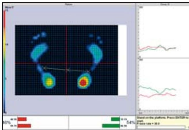
The measurements and the evaluation are processed on the computer using the WinFDM program. For this procedure, the measuring data of the floor reaction forces, the video camera and, if applicable, the EMG and angle data are evaluated synchronously. The measurements may be observed in the "Viewer" and rate of playback may be adjusted.
