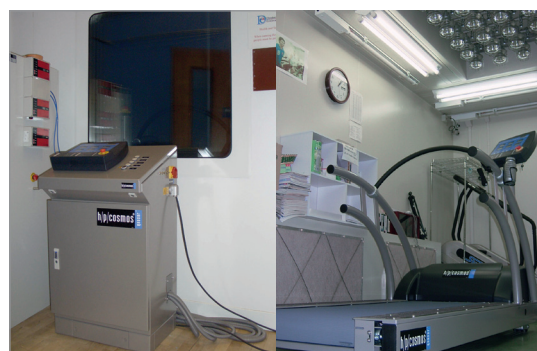
environmental chamber installation with remote control
